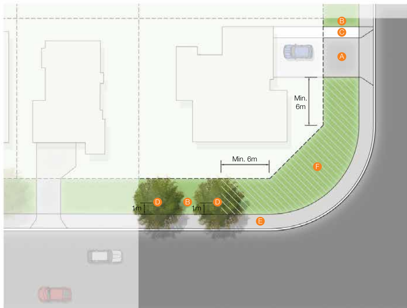
FIGURE 4: Typical corner verge layout with footpath
