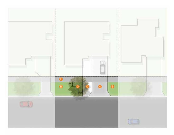
FIGURE 2: Typical verge layout with footpath
