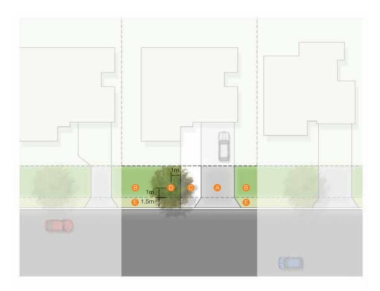
FIGURE 1: Typical verge layout without footpath
