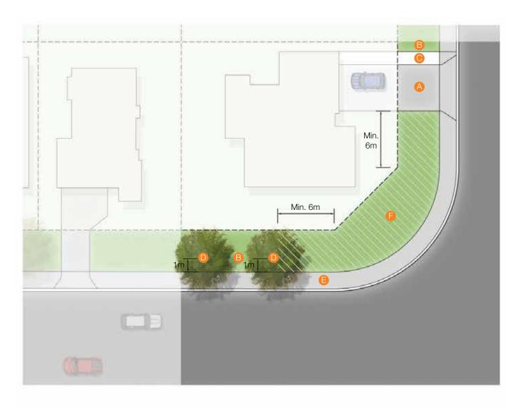
FIGURE 4: Typical corner verge layout with footpath
