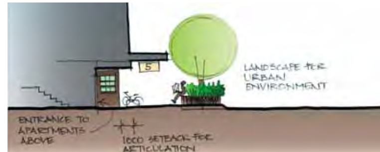
Figure 26. Active Facade Articulation (mixed use)
