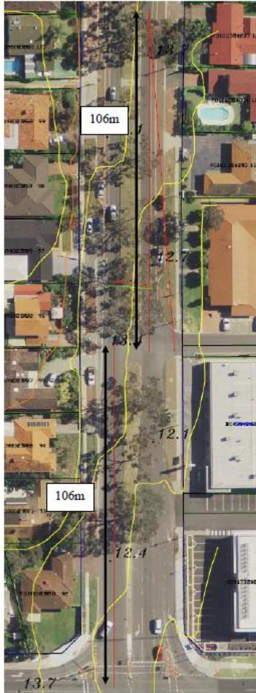
Figure 3: Minimum SISD for the northern driveway crossover
