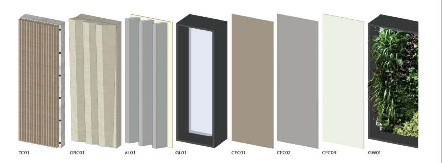
TC01 - TIMBER CLADDING 55mm CENTRES 100x25m PROFILE GRC01 - GLASS REINFORCED CONCRETE MOULDED PANELS (SANDBLASTED) AL01 - ANODISED ALUMINIUM FINS (COLOUR INDICATVE)GL01 - GLAZING WITH POWDERCOATED ALUMINUM FRAME CFC01- FIBRE CEMENT PANEL COLOUR 1 CFC02- FIBRE CEMENT PANEL COLOUR 2 CFC01- FIBRE CEMENT PANEL COLOUR 3 GW01 - PANELISED GREEN WALL SYSTEM
