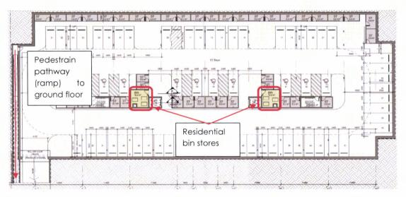
Figure 1: Basement plan showing two bin stores including chutes & pedestrian pathway for transfer of bins to ground floor
