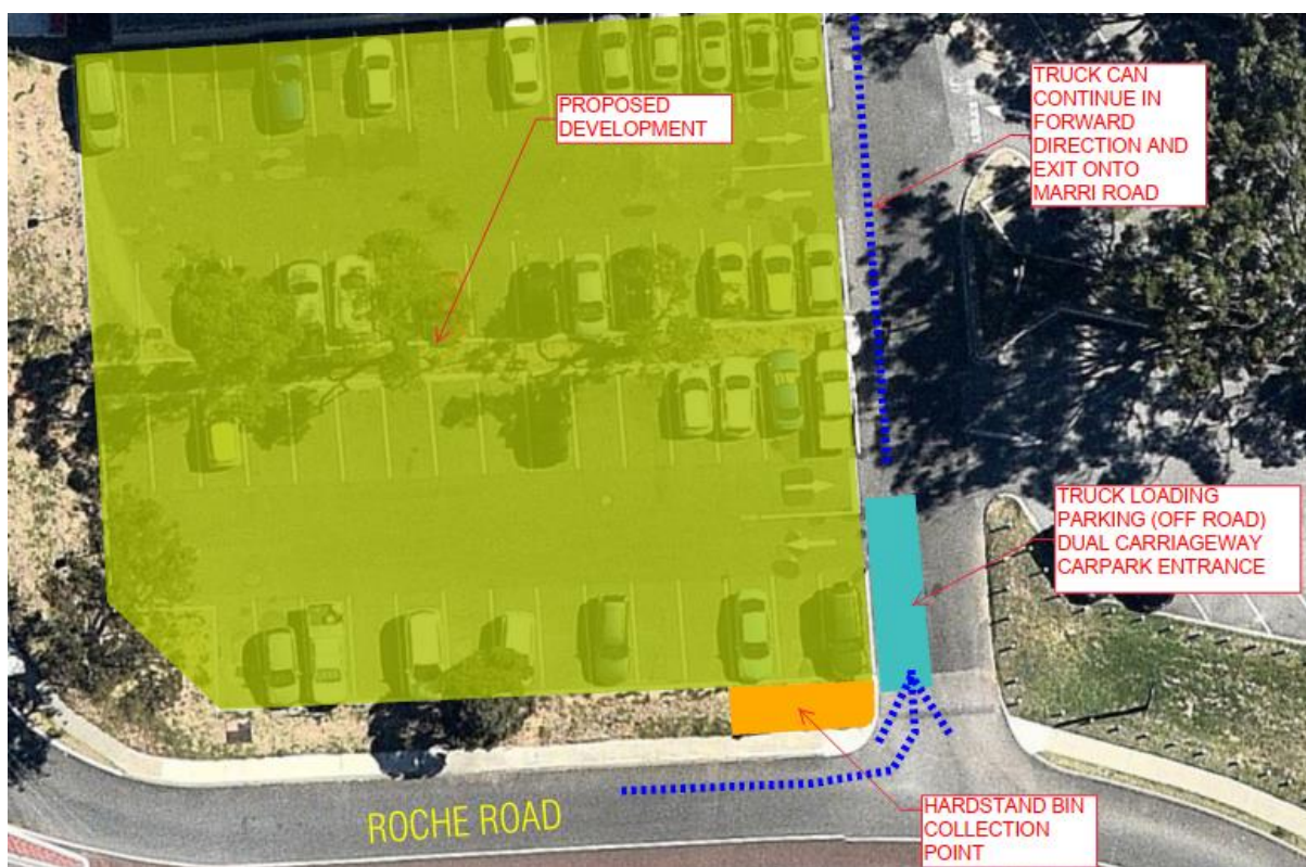
Figure 2: ground floor plan showing waste collection route.
