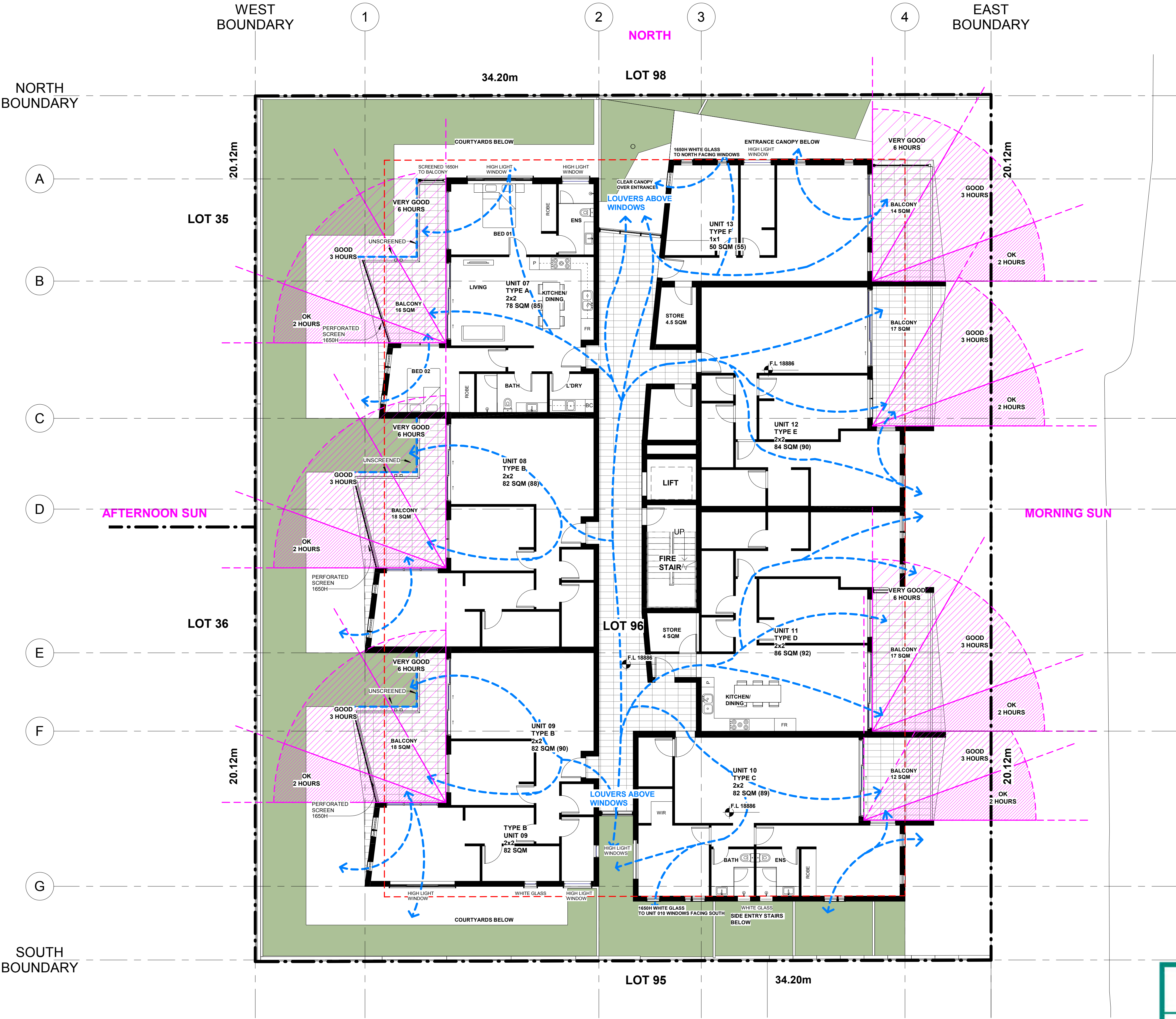
1 SOLAR ACCESS & CROSS VENTILATION DIAGRAM - FIRST FLOOR 1 : 100
