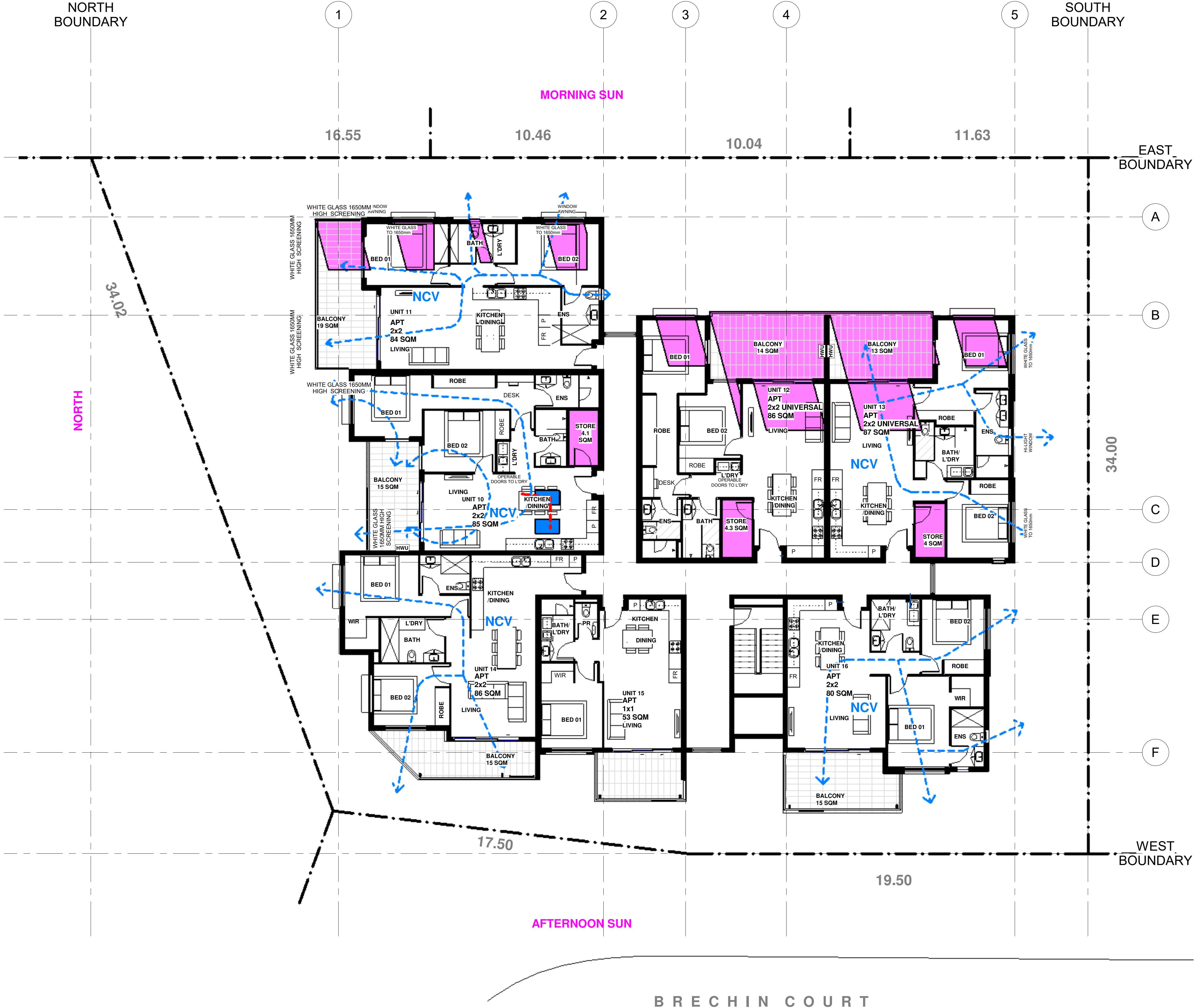
SOLAR ACCESS & CROSS VENTILATION DIAGRAM - SECOND FLOOR - 9-00 SUN
