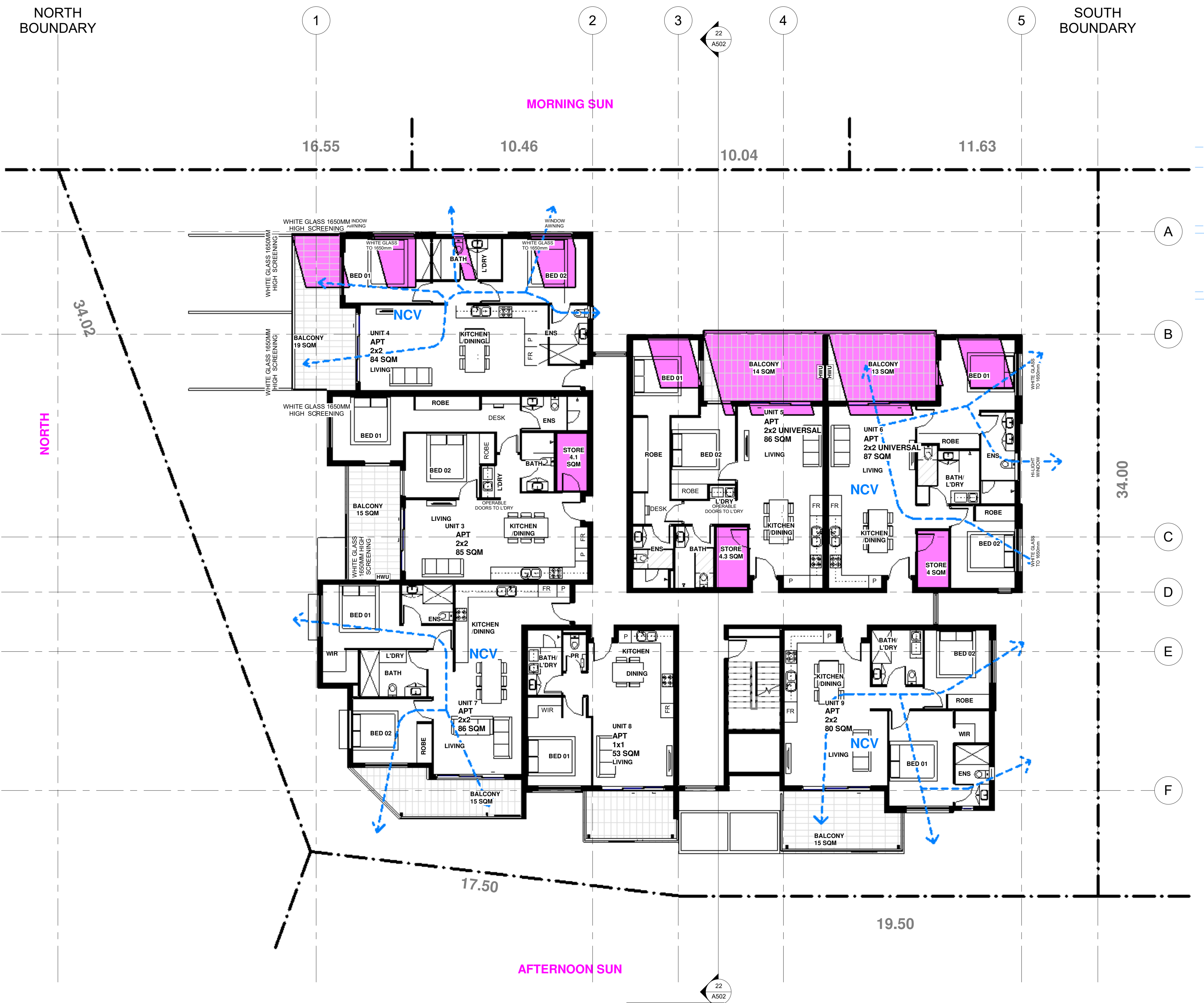
SOLAR ACCESS & CROSS VENTILATION DIAGRAM - 9-00 SUN 1 : 100
