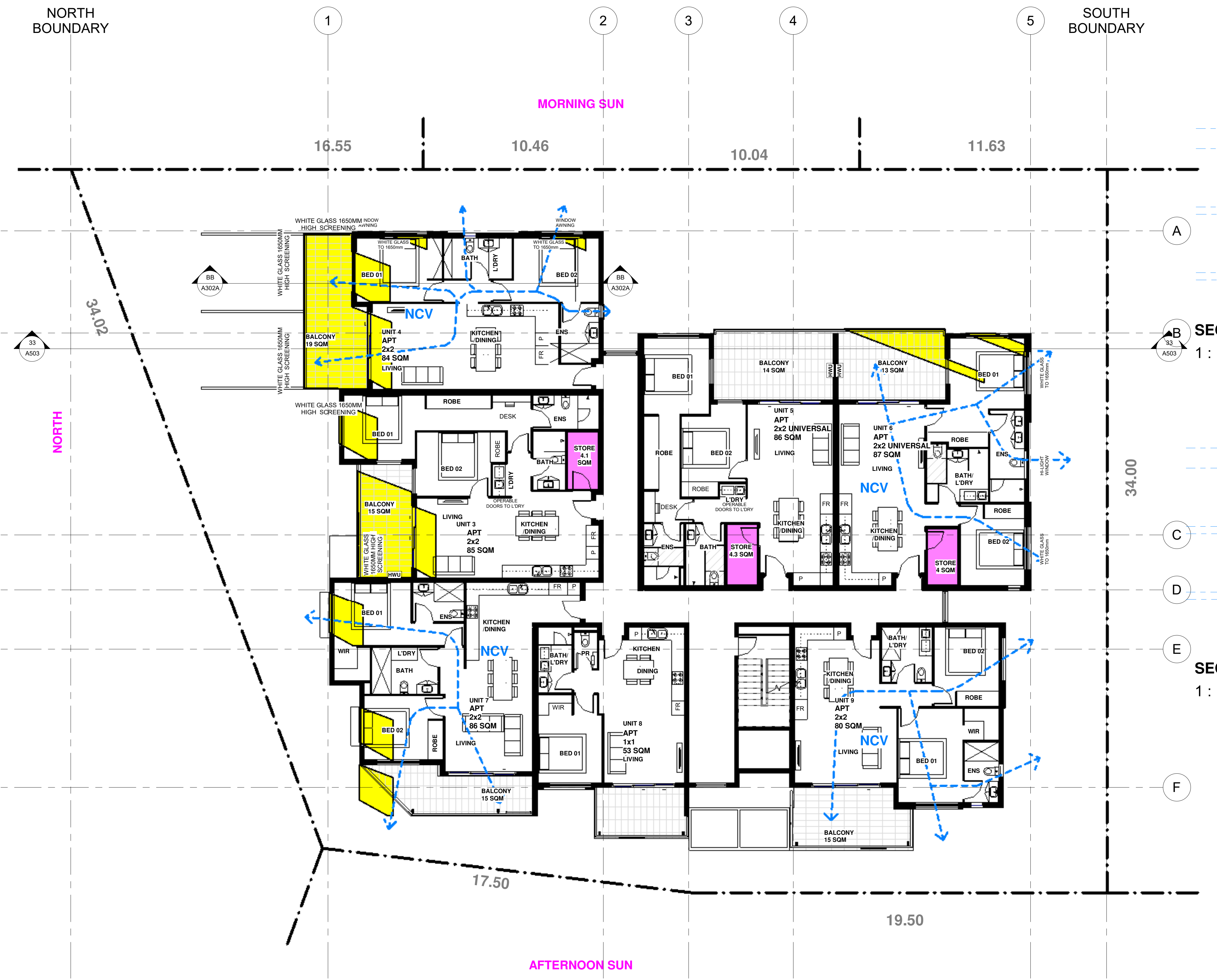
SOLAR ACCESS & CROSS VENTILATION DIAGRAM - FIRST FLOOR - 12:00 SUN
