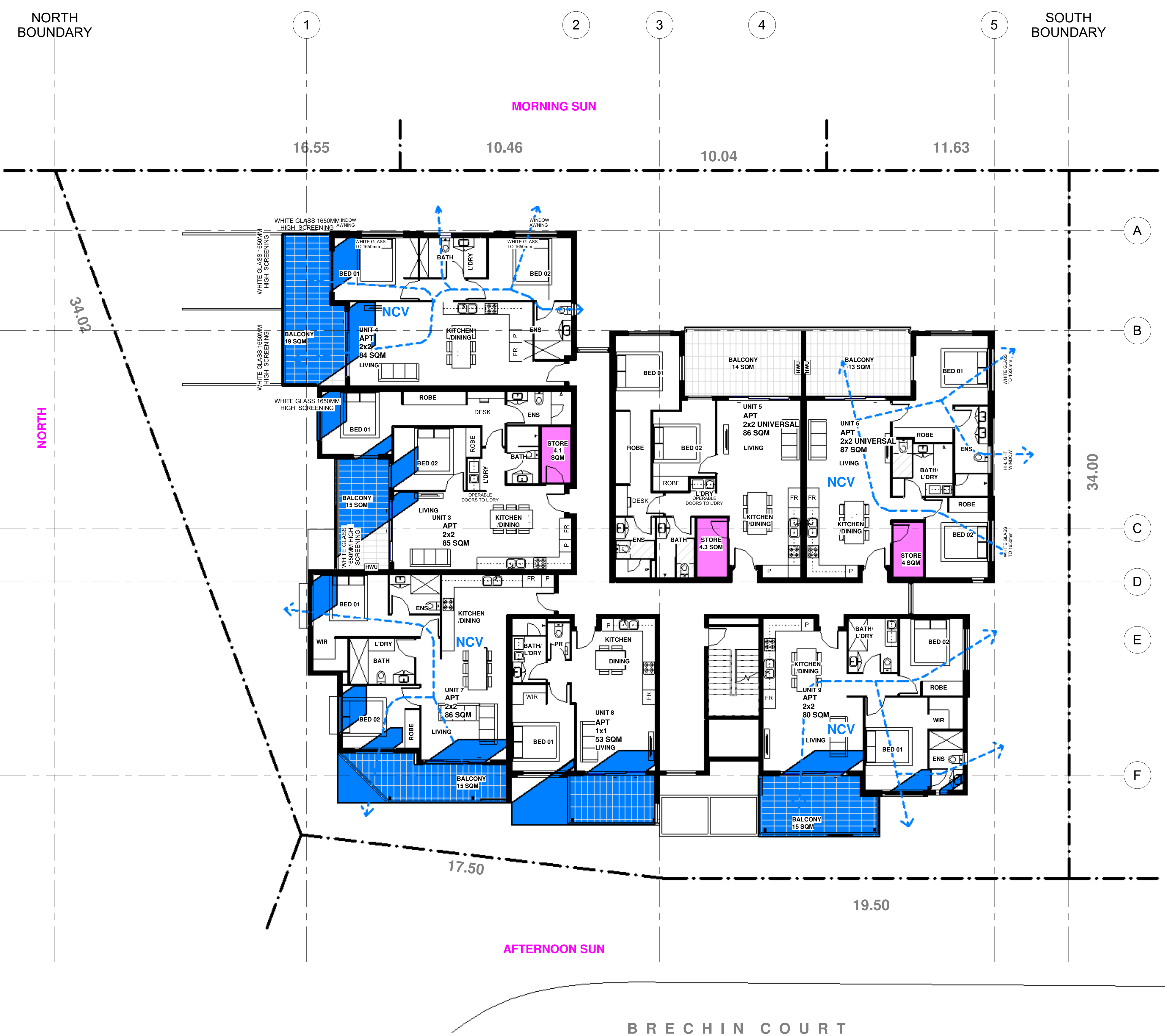
SOLAR ACCESS & CROSS VENTILATION DIAGRAM - 15-00 SUN
