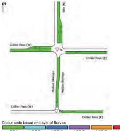
LOS A LOS B LOS C LOS D LOS E LOS F Delay model settings are specified for individual Sites forming the Network.
