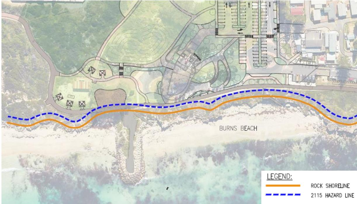
**Figure 3.1 Coastal Erosion Hazard Line**
