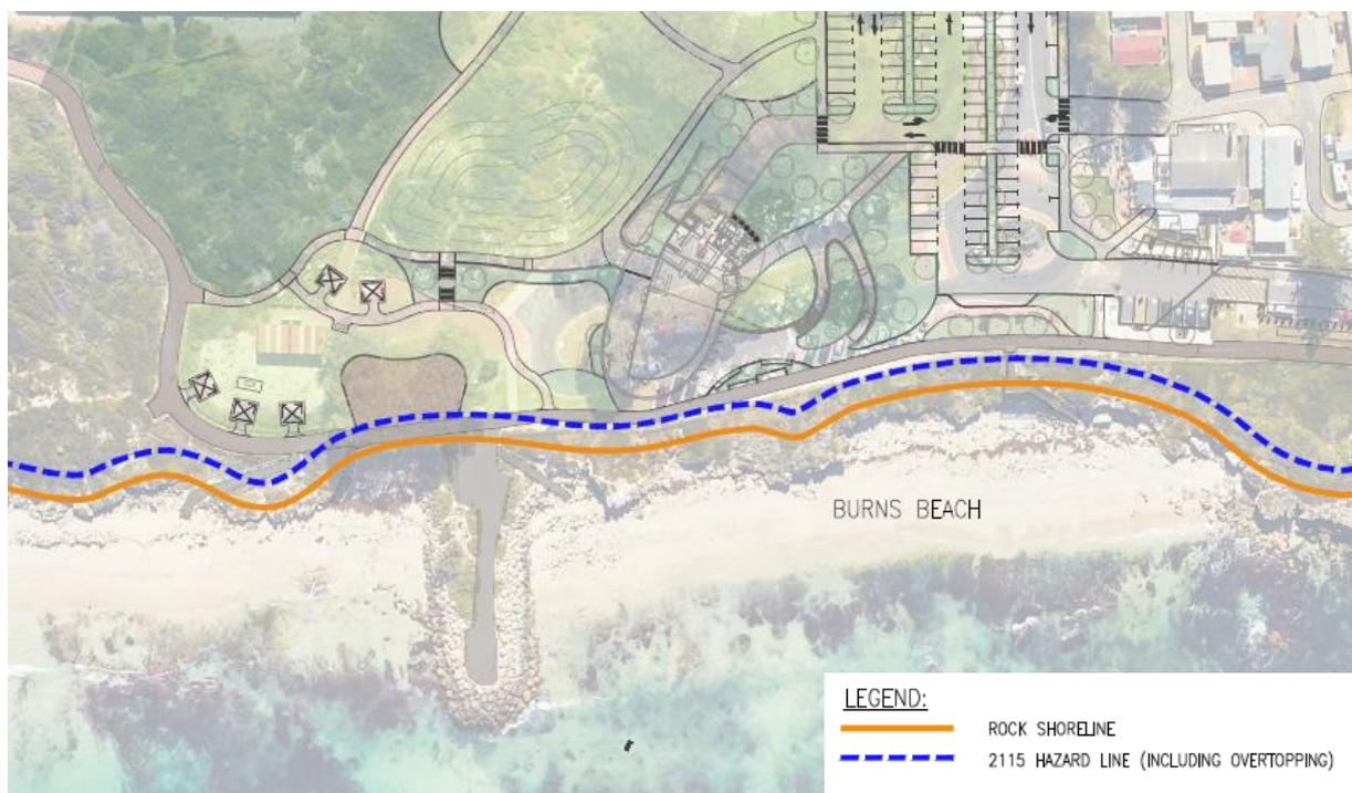
**Figure 5.1 Wave Overtopping Hazard Line**
