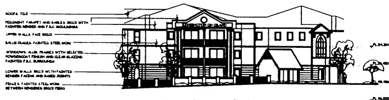
Crn Grand Boulevard & Shenton Avenue Elevation
