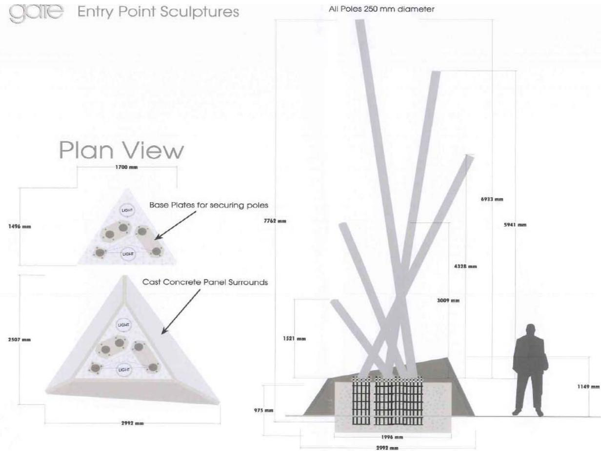
Concrete footing with cage partially underground steel structure is bolted onto cage via base plates
