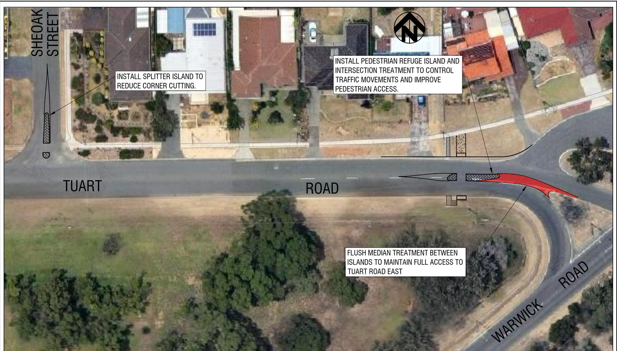
INSTALL SPLITTER ISLAND TO REDUCE CORNER CUTTING.
