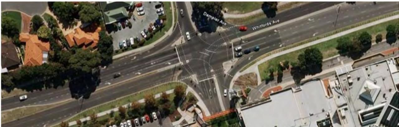
**Whitfords Avenue/Marmion Avenue** – A major 4-way signalised intersection including right turning pockets and left-turn unsignalised slip lanes on all approaches. The existing layout of this intersection is shown in Figure 5-9. Pedestrian provision has not been explicitly included within the signal phasing; however actuated crossing facilities are provided. Long red phases for all approaches provide sufficient crossing time for pedestrians intending to cross at this location.
