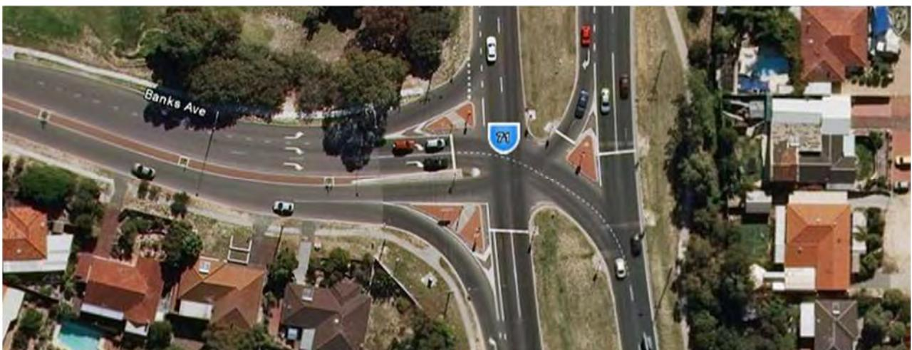
**Marmion Avenue/Cook Avenue** – A 3-way priority controlled intersection including a right turning pocket and left turn slip lane on Marmion Avenue, as shown in Figure 5-11. The seagull island within the central median allows for staged crossing for right-turning traffic, with sufficient space for queuing of up to two cars. This significantly improves traffic operations for right-turning vehicle movements.
