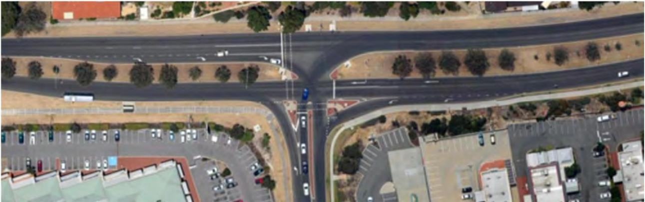
**Whitfords Avenue/Dampier Avenue/shopping centre access** – A 4-way signalised intersection including left and right turning pockets on Whitfords Avenue as shown in Figure 5-8. Provision for crossing pedestrians is explicitly included within the signal phasing.
