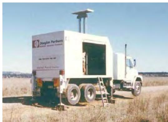
Figure 2: Purpose built CPT rig
