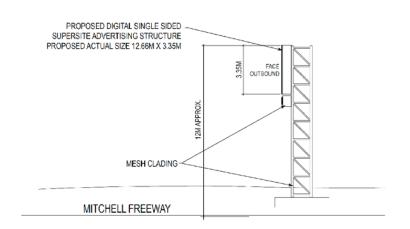
NORTH ELEVATION WEST ELEVATION
