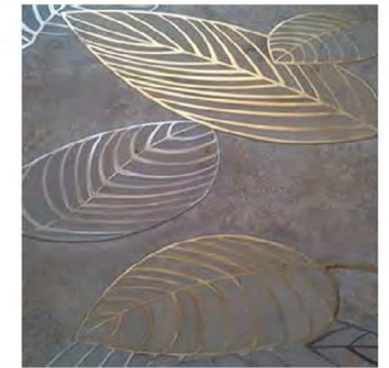
Example of steel inlay in concrete
