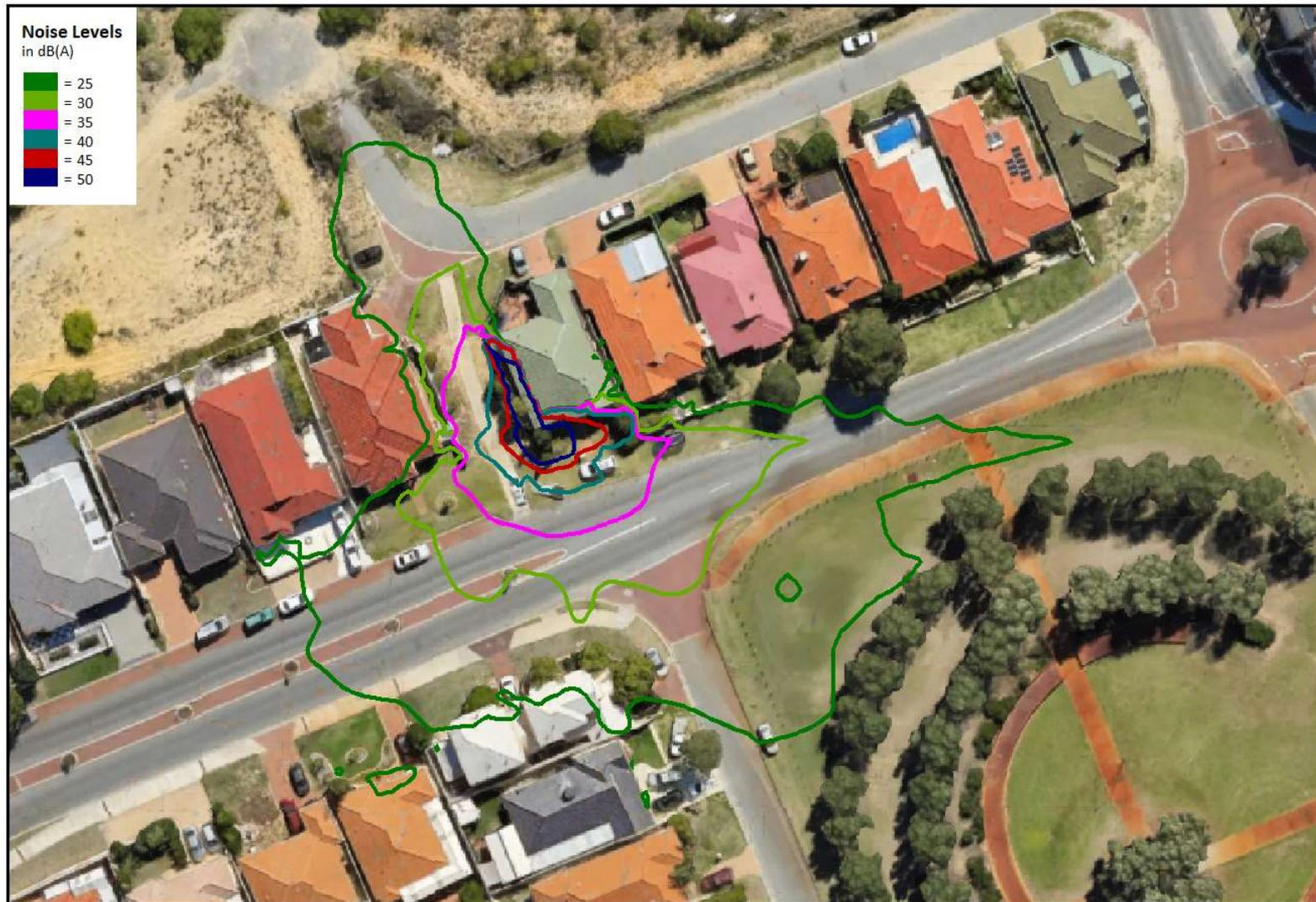
**Figure 6: Worst-case noise level contour for scenario 1.**
