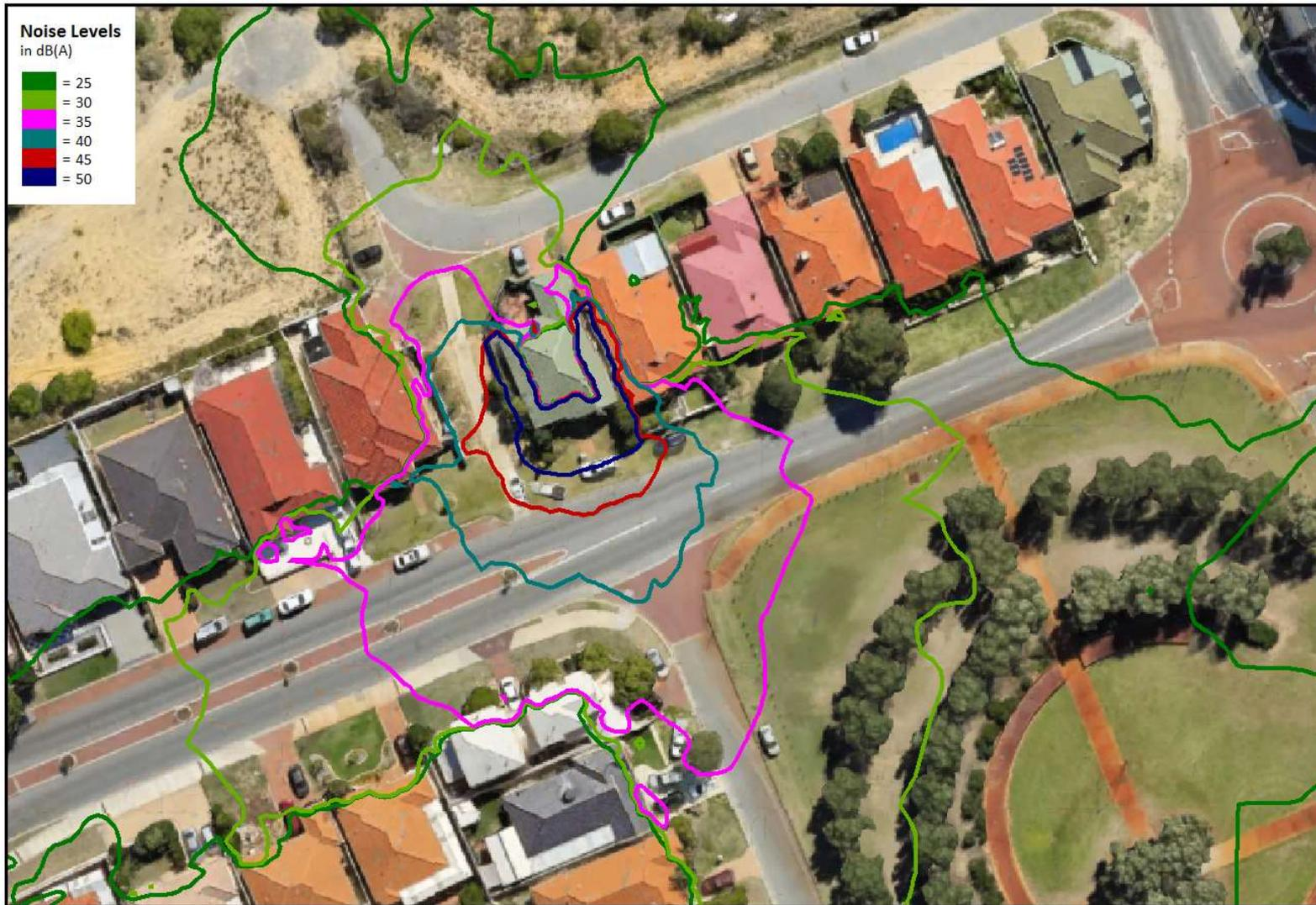
**Figure 7: Worst-case noise level contour for scenario 2.**
