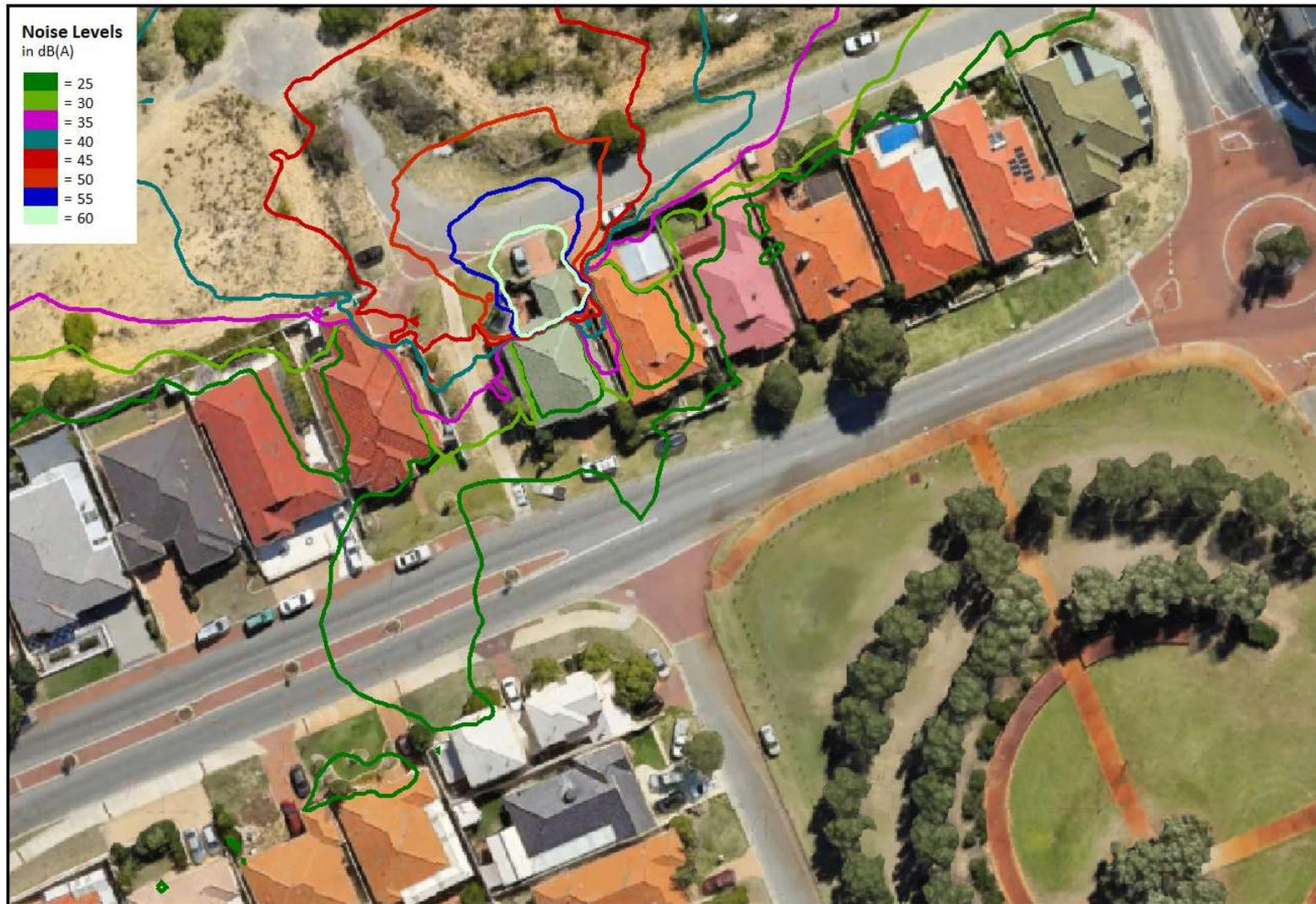
**Figure 9: Worst-case noise level contour for scenario 4.**
