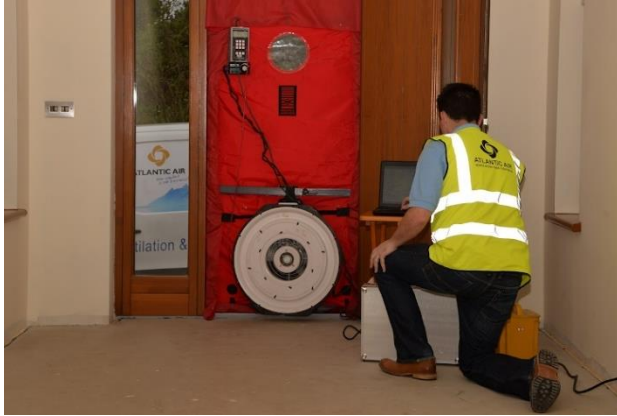
Figure 10.1 - Example of airtightness testing
