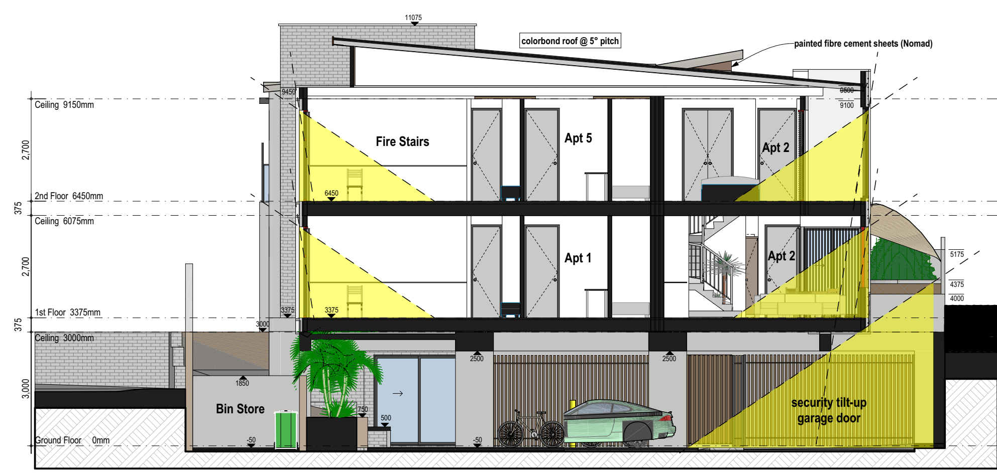
S2 Section / Solar Access 1:100
